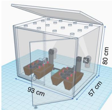
Figure 1. Drawing of environmental chamber
